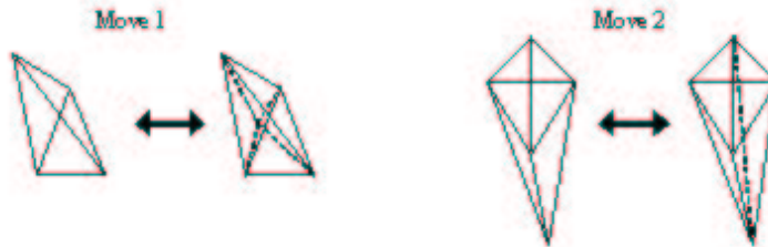
FIGURE 4.1. Local triangulation moves. Left: Splitting one tetrahedron into 4 by adding a central vertex, or vice versa. Right: Two tetrahedra glued along their base change into 3 tetrahedra with sides glued along the dashed line, or vice versa.
